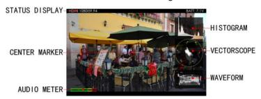
Figure 5-2 Tools for G7 4K ULTRAHD Monitor
