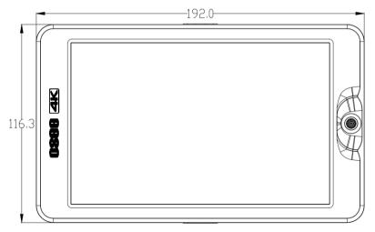
Figure 7.2-1 Front View(Unit: mm)
