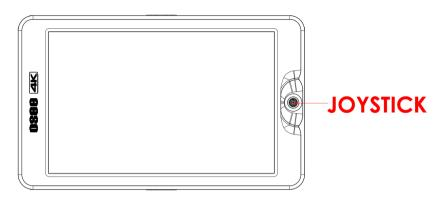
Figure 4.2-1 Buttons in Front Panel
