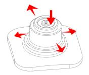
Figure 4.3-1 Five Operation Directions for Joystick
