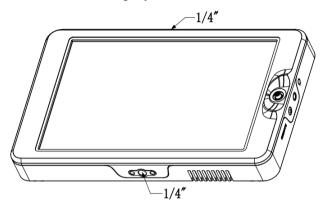
Figure 3-4 Positions for Hanger Installation
